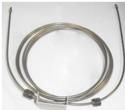
PACKED COLUMN FOR GAS CHROMATOGRAPHY
